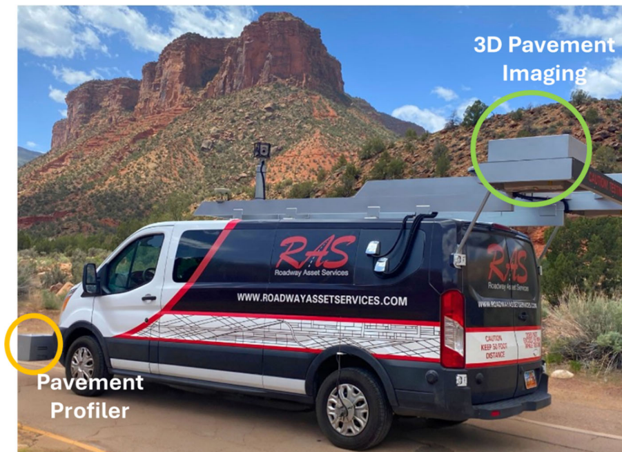
Figure 5. RAC pavement condition data collection system.
