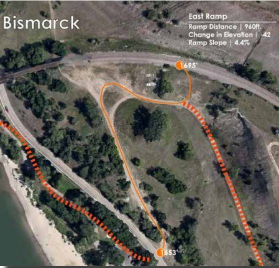
[figure 11.2] east ramp connection
